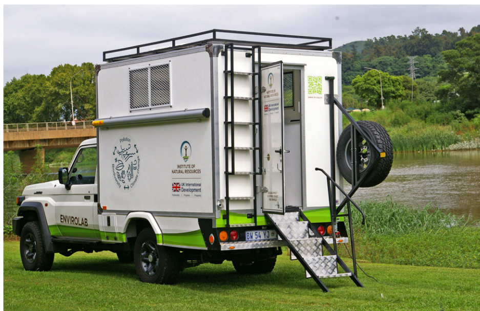
The new ENVIROLAB is a mobile water testing unit funded by Defra.
